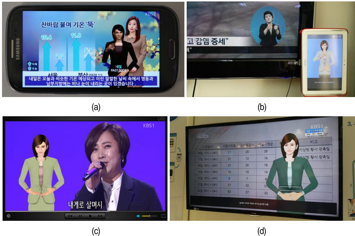
Figure 6 – Demonstration of the proposed system. (a) Weather forecast application, (b) mobile application for real-time sign language interpretation, (c) PC software playing video and script files at offline mode, (d) the output of the PC software (online mode) composited on the live TV screen using a chromakeyer.
