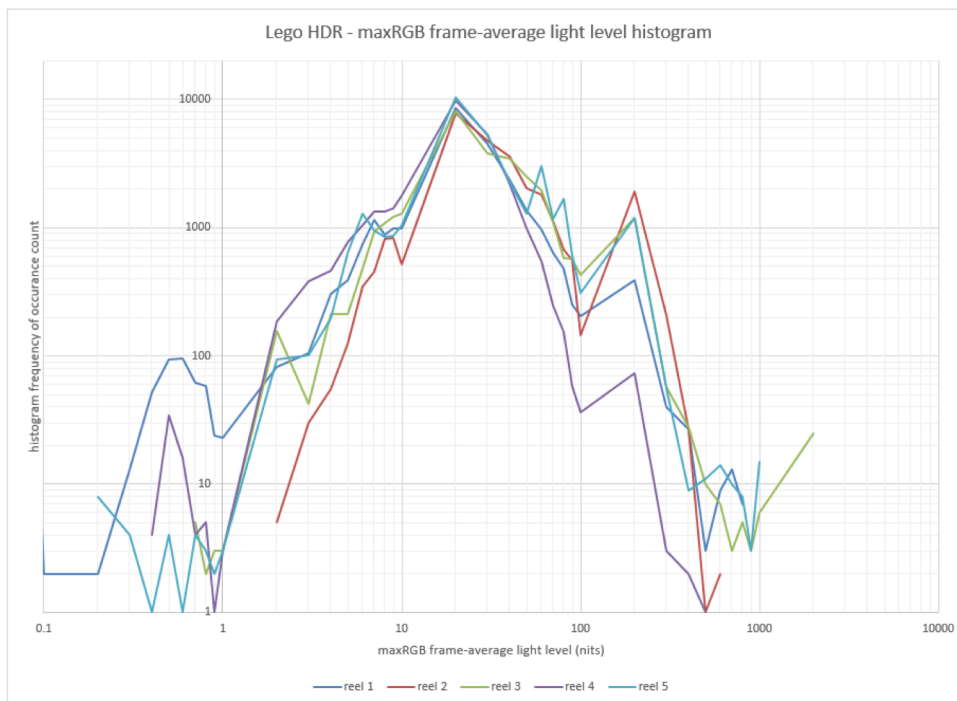
Figure 2 – Histogram of Frame-Average Light Levels for the entire “Lego Movie” (Reel 1 through 5).
