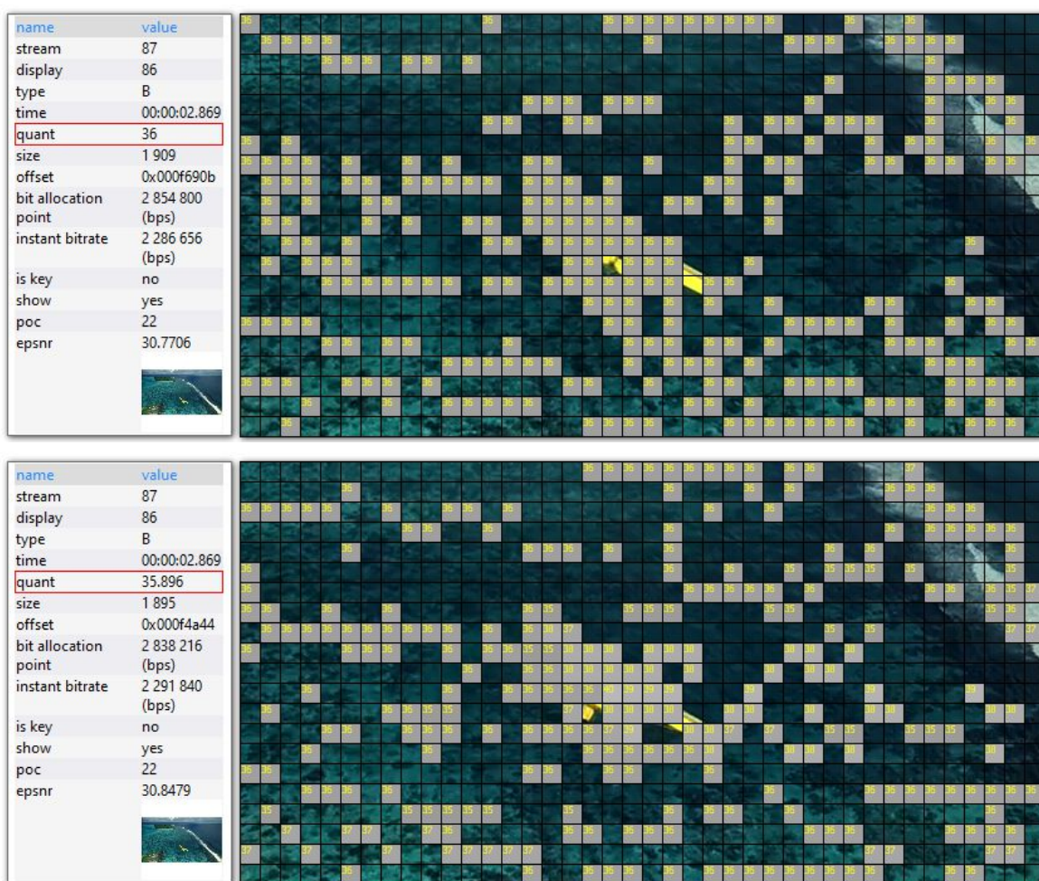
Fig. 14 Values of constant (above) and adaptive (below) quantizers for one and the same frame.
