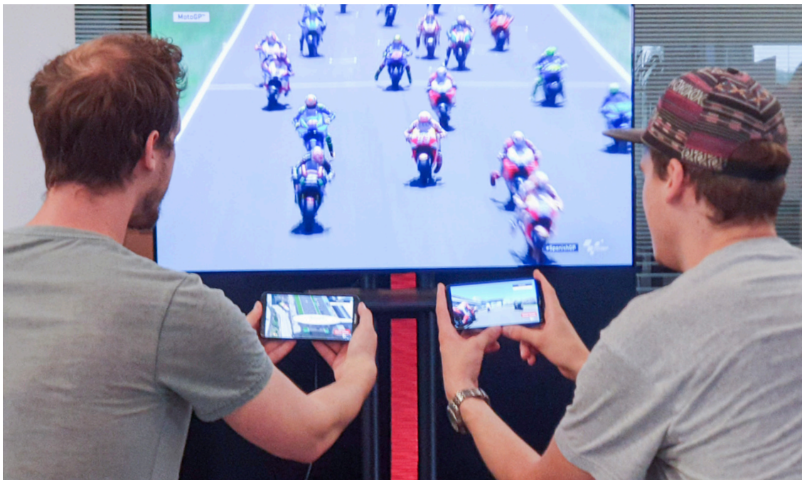
Fig 1: Large screen showing the main programme and two 'second screens' showing personalised content, merged together using Hybrid Multiview Broadcast .
