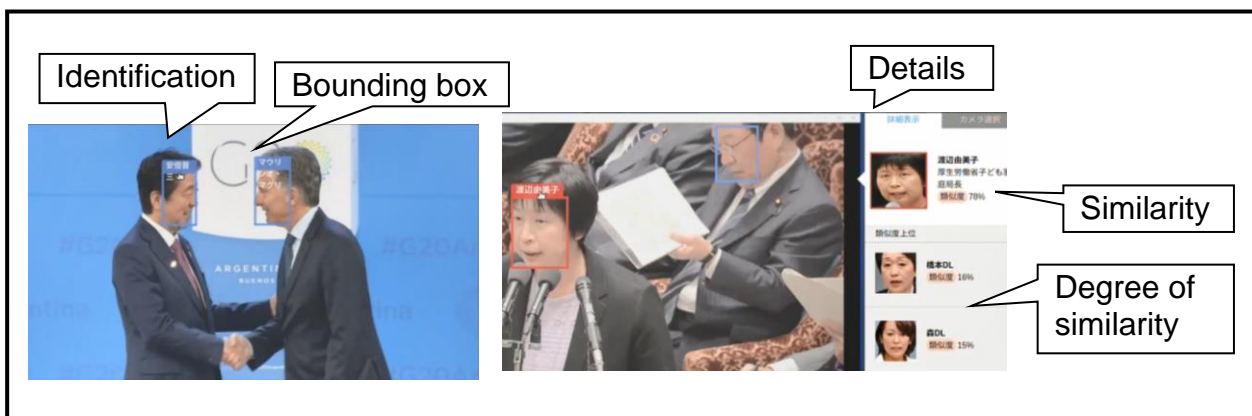
Figure 1 - Example showing how Face Detector works
