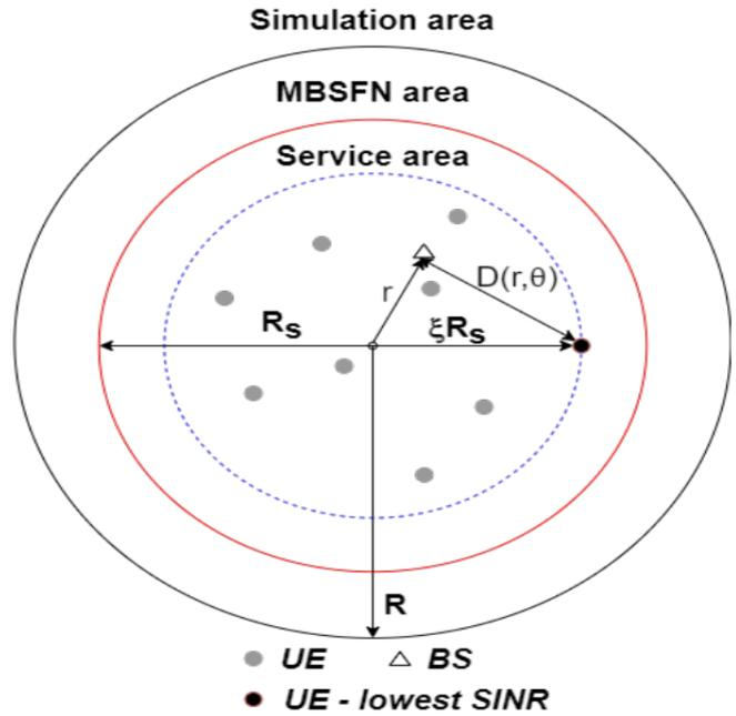
Figure 4 - Model for the MBSFN SINR distribution
