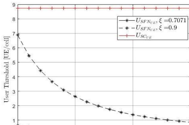
Figure 6 - User threshold to switch from unicast to MBSFN or SC-PTM in order to reduce energy consumption in the BS or UE.
