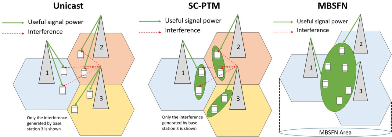
Figure 2 - Unicast and broadcast transmission modes
