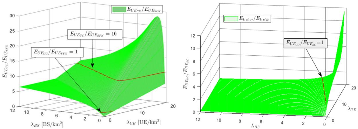
Figure 5 - Ratio between the UE energy consumption in UC and MBSFN modes (left). Ratio between the UE energy consumption in UC and SC-PTM modes (right).
