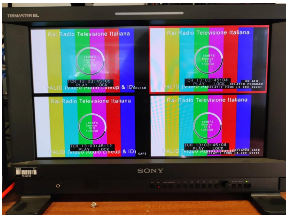
Figure 7 – Synchronization tests: two inputs (top and bottom left) and the two synchronized outputs (top and bottom right)
