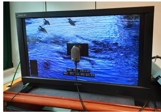
Figure 8 - A frame of the video used for latency measurement and the photodiode
