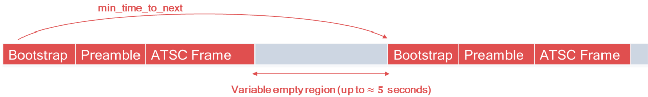
Figure 3: Illustration of the ATSC 3.0 Frame Structure, facilitating gaps between successive bootstrap signals.
