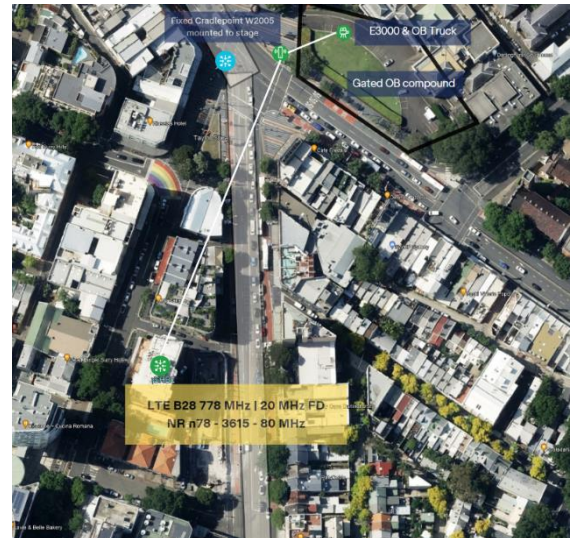
Figure 5 - Installation position and bearing to serving cell
