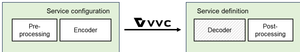
Figure 1 - Encoder-decoder video flow and scope of VVC technical guidelines.
