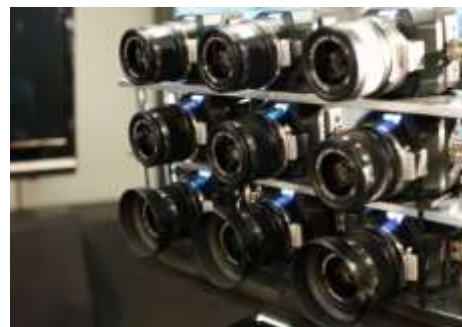
Figure 3 – 3x3 camera array built from Black Magic Micro Studio 4K cameras.
