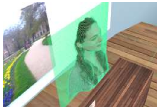
Figure 8 –.The lightfield as seen from an extreme position. Depth from the lightfield is mapped on the canvas element forming an approximate 3D hull. This hull can be used to recover approximate normal maps for correct handling of CG-lighting.
