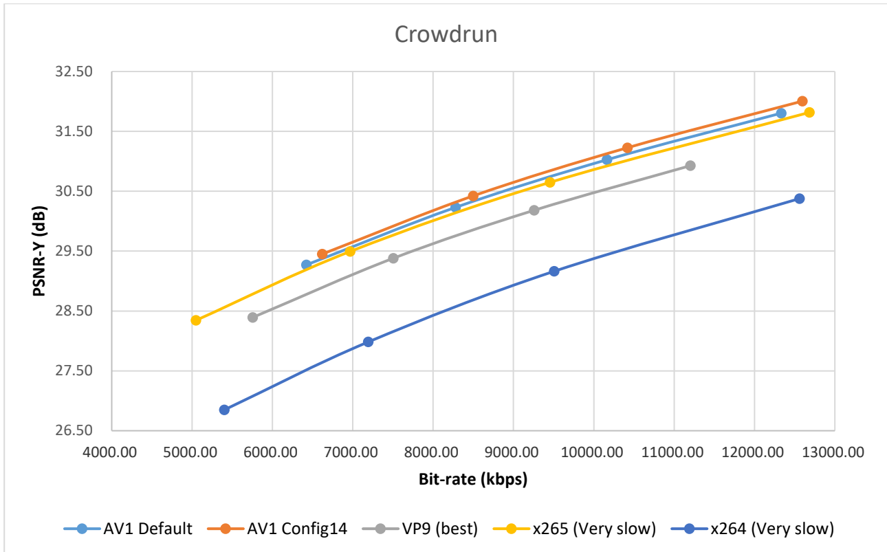
Figure 2b: Rate-Distortion plots for Crowdrun-1080p@50fps sequence
