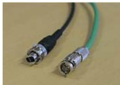
Figure 15– U-SDI (left) and coaxial (right) cables
