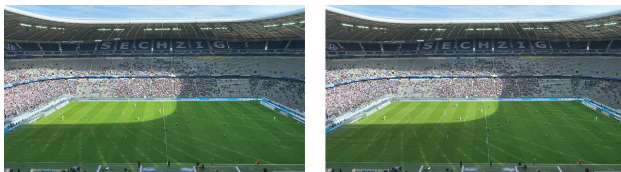
Figure 8 – The left image shows the tone mapping in XYZ, the right one in IPT. The grass and the sky in XYZ have a little hue shift and look more burned-out.
