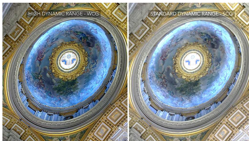
Figure 13 – Indoor pictures acquired (HDR HLG BT.2020 on left and SDR BT.709 on right)
