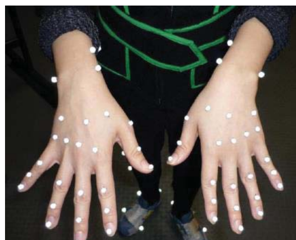
Figure 2 – Markers attached to the fingers for an optical motion capture
