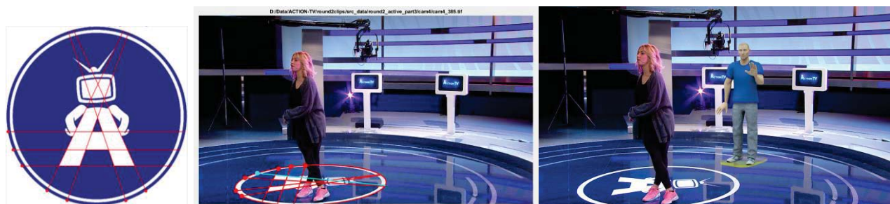
Figure 5 – ACTION-TV logo (left), detected features in the camera view (middle) and perspective correct rendering of virtual candidate (right)
