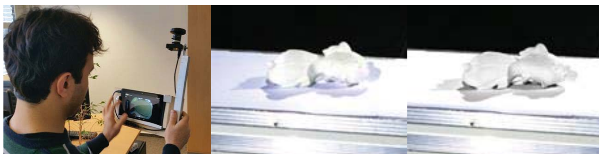
Figure 6 - Light probing device (left), image of reference object (middle) and rendered image of the object with estimated lighting (right)
