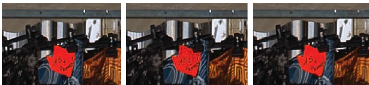
Figure 3 – Chroma leakage example. Original (left), Conventional 4:2:0 (middle) and 4:2:0 with luma adjustment (right). Sequence courtesy of Technicolor and the NevEx project.
